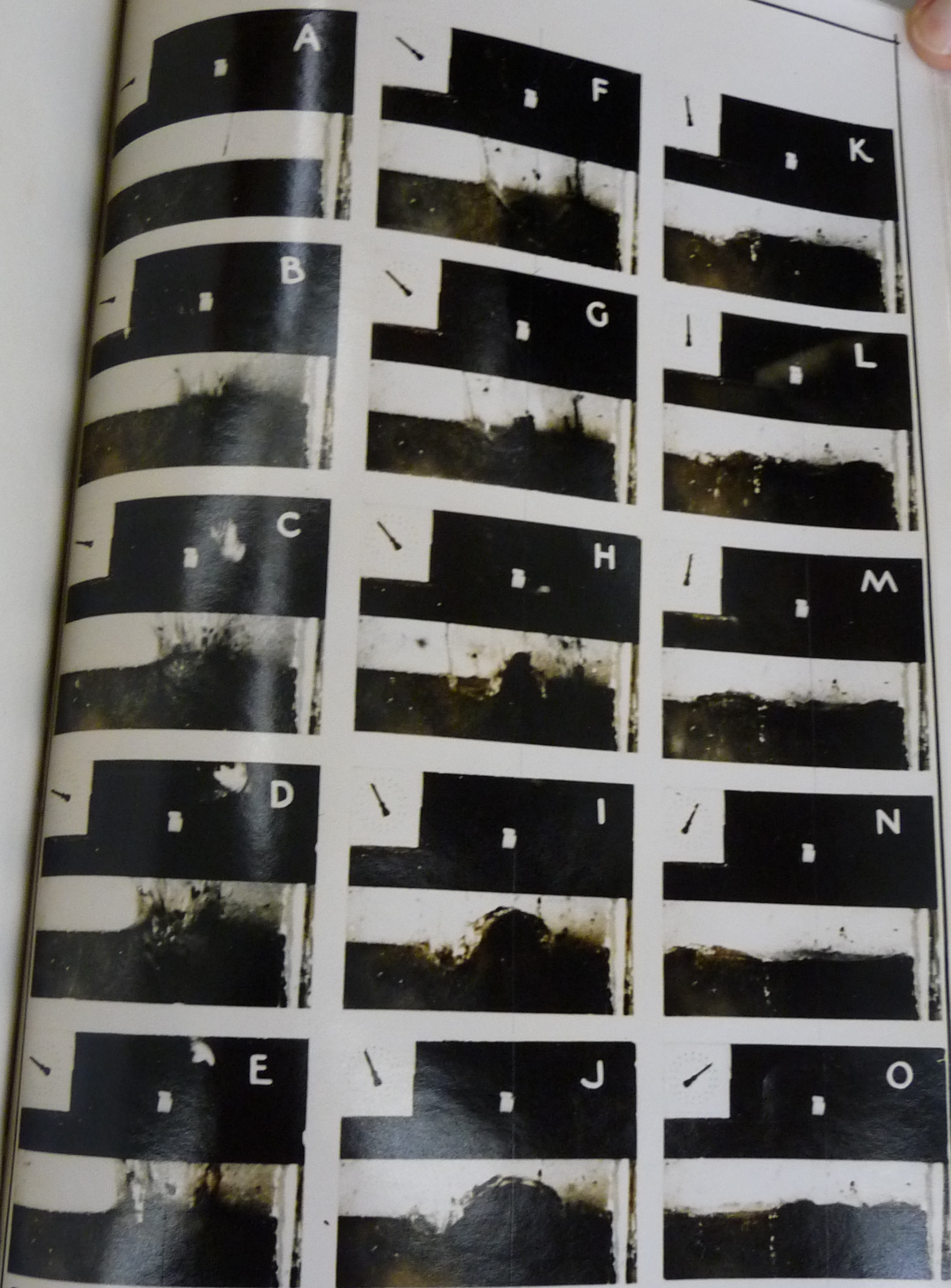
Successive Photographs of the initiation of an approximately two-dimensional wave train by means of a fire cracker.
