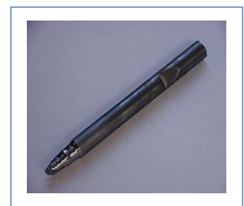
A puller rod with seed crystal for growing single-crystal silicon by the Czochralski process
